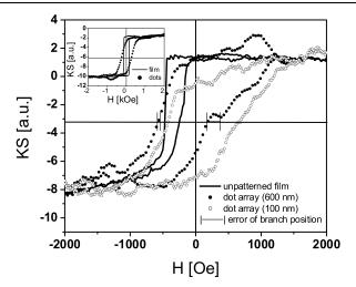
FIG. 2. MOKE signal (KS) of  $M_l$  vs H of unpatterned Fe-FeF<sub>2</sub> film and different Fe dot arrays on FeF<sub>2</sub> at 10 K (below  $T_N$ ). The inset shows the signal of unpatterned Fe-FeF<sub>2</sub> film and the 600 nm Fe dots on FeF<sub>2</sub> at 90 K (above  $T_N$ ).
